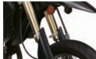
Motocrosser-derived inverted front forks
